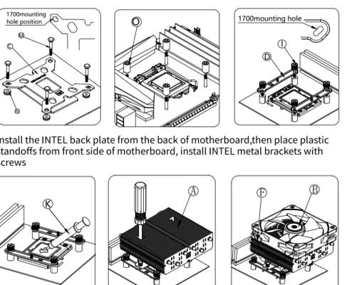
Install the INTEL back plate from the back of motherboard, then place plastic standoffs from front side of motherboard, install INTEL metal brackets with screws
