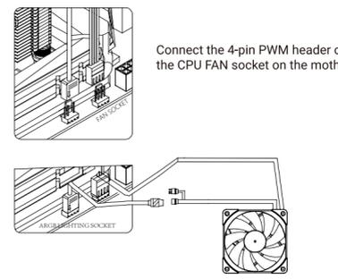
Connect the 4-pin PWM header of fan into the CPU FAN socket on the motherboard.
