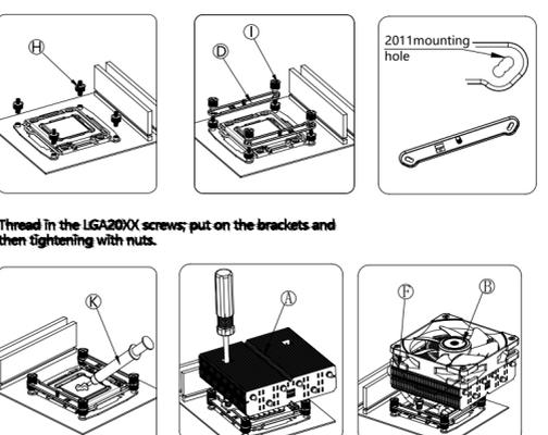
Thread in the LGA20XX screws; put on the brackets and then tightening with nuts.
