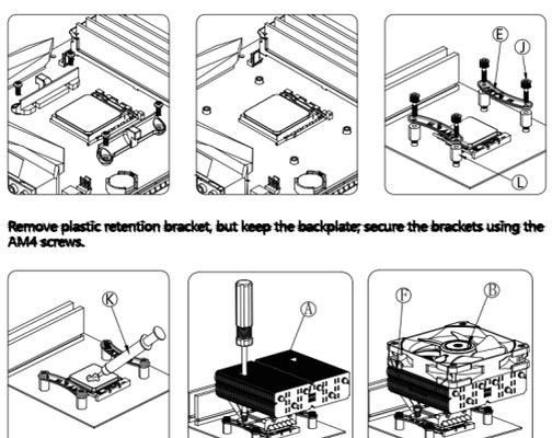
Remove plastic retention bracket, but keep the backplate; secure the brackets using the AM4 screws.
